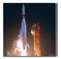
• **Cause:** A programmer incorrectly transcribed a handwritten formula into computer code, missing a single superscript bar. Without the smoothing function indicated by the bar, the software treated normal variations of velocity as if they were serious, causing faulty corrections that sent the rocket off course.
