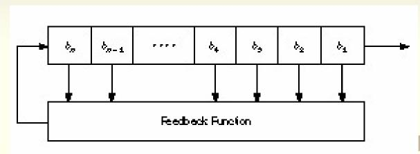
Figure 16.1 Feedback shift register.
